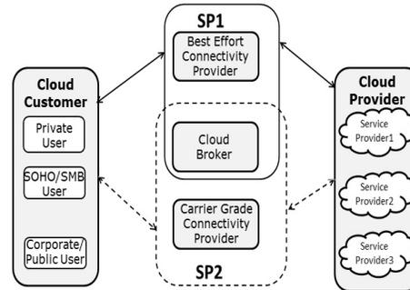
Figure 1. Supplementing best effort connectivity for SaaS brokering with carrier grade connectivity
